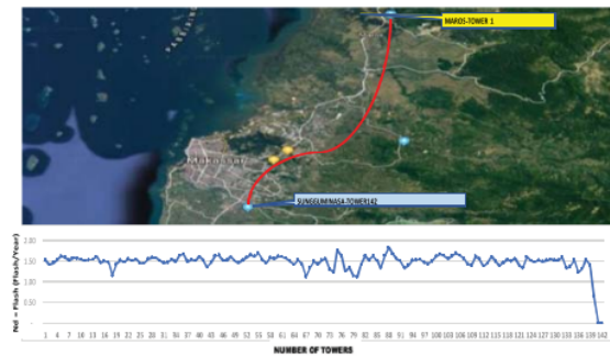
Fig. 1. Geographical Profile of Tower 150 kV Lines [2]
